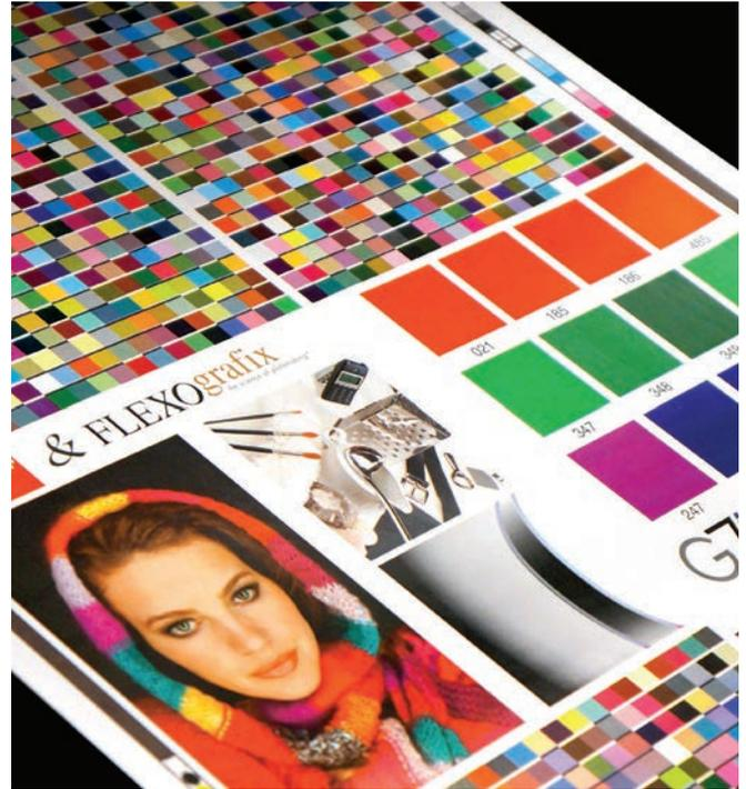
Profile test using a set of plates with the curve applied from the fingerprint
