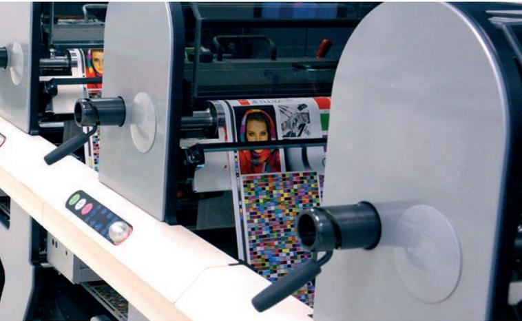
Key parameters to control include registration, impression and drying/curing
